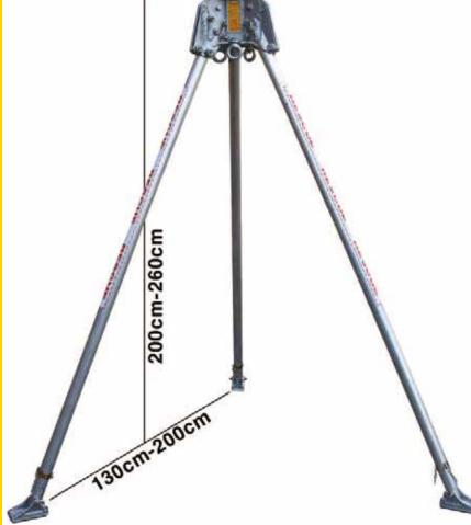
The RT3 has 6 anchor points tested to EN795. The 3 overhead pulleys hold up to 11mm rope. The extra swivel anchor points may be used with pulleys for a double roped rescuer, back-up system, airlines, communication lines, medical kits, tools etc.
