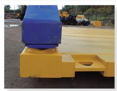
Connect the assemled plates with each other by screwing the rolling struts together.
