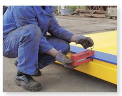
Fit the plates with the lower limit pins. Put on the rolling struts, push them against the limit pins and fix them with the upper limit pins.
